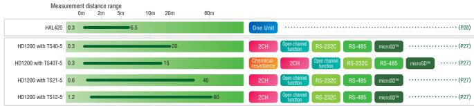
Please select the model that the desired measurement distance is around the middle of covering range.
