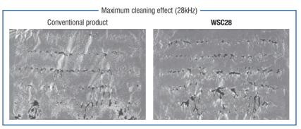
FM + AM oscillation with our original transducer enables to improve transmission efficiency of ultrasound. As the a result, higher cleaning power is achieved at low power consumption.
