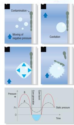
appearing that cavitation is like crawling on vibration surface, ultrasound is not effectively generated, and also deterioration of vibration board to cause erosion is accelerated. Changing liquid deepness makes cavitation generation effective and ultrasonic cleaning effective, too.
