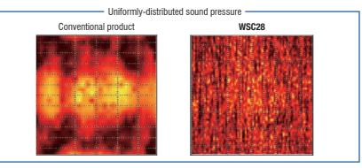
Cavitations can be distributed both with FM and AM modes in the cleaning tank so that uniformity of cleaning can be improved.
