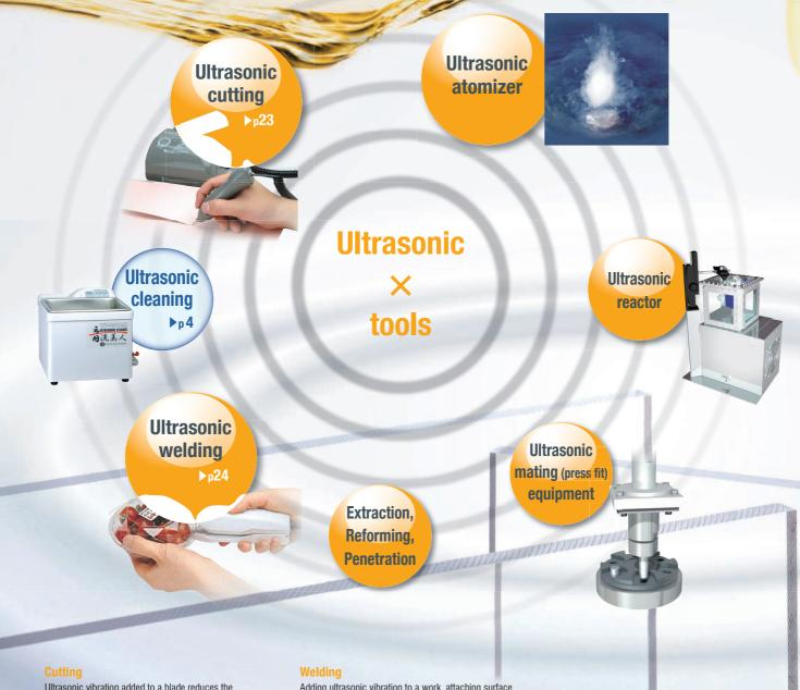
Ultrasonic vibration added to a blade reduces the friction towards the object and cutting ability extremely increase (acceleration).
