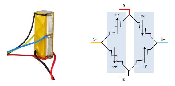
The induced differential voltage  $V_S$  for a two-varying element full bridge is [1, 2]
