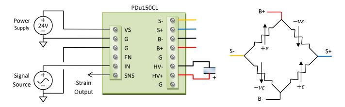
After connection, the module is calibrated so that a full-range extension of the actuator produces a +10V sensor output. The module can then be switched to closed-loop where a 0V to 10V input produces a zero to full-range extension of the actuator.
