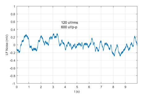
Figure 3. Low frequency noise from 0.03 Hz to 20 Hz
