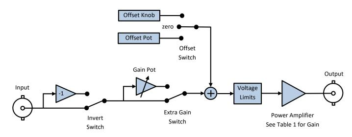
Figure 5. Signal path with switches in default positions.
