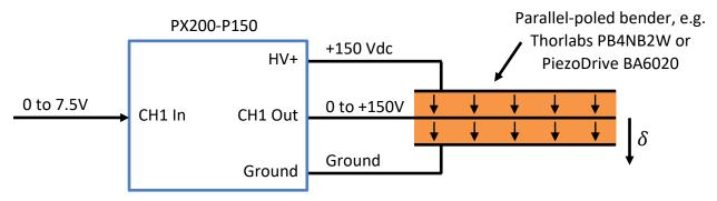
Figure 6. Parallel-poled bender driven in the biased unipolar configuration [1].
