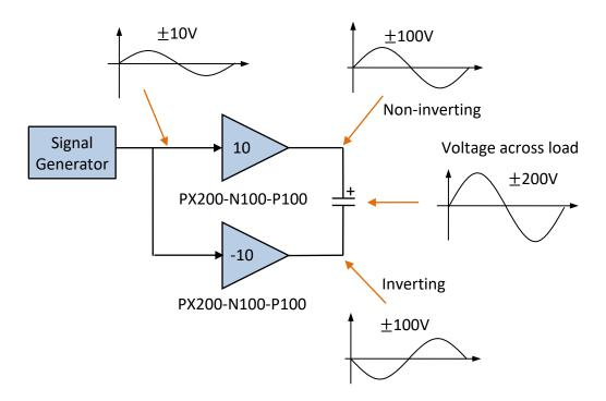
Figure 8. Bridge mode configuration for obtaining  $\pm 200V$
