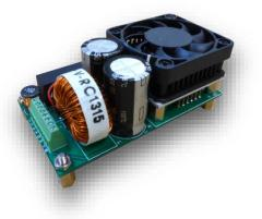
The MX200 is a complete power supply and highperformance linear amplifier module for driving piezoelectric actuators. The MX200 can drive stack actuators; standard piezoelectric actuators; two wire benders; and three-wire piezoelectric benders requiring a bias voltage. Output currents of up to 1 Amp are developed at frequencies up to 100 kHz with less than 100 uV noise (10Hz to 10kHz). Bipolar output voltages up to +/-100V are possible with an external AC coupling capacitor.
