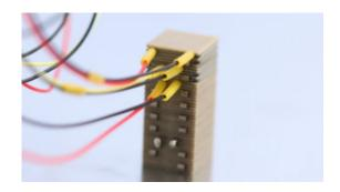
The Noliac shear stack NAC3404-H12.6 features motion in the X/Y/Z-axis. NAC3404-H12.6 measures 15x15 mm with a height of 12.6 mm and provides free stroke of 3/3/3  $\mu$ m and a capacitance of 14.9/14.9/92.8 nF.
