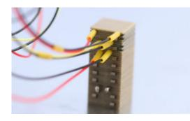
The Noliac shear stack NAC3403-H23.1 features motion in the X/Y/Z-axis. NAC3403-H23.1 measures 10x10 mm with a height of 23.1 mm and provides free stroke of 6/6/6  $\mu$ m and a capacitance of 13.3/13.3/85.4 nF.
