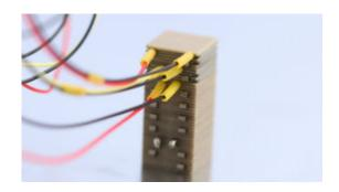
The Noliac shear stack NAC3403-H12.6 features motion in the X/Y/Z-axis. NAC3403-H12.6 measures 10x10 mm with a height of 12.6 mm and provides free stroke of 3/3/3  $\mu$ m and a capacitance of 6.6/6.6/42.7 nF.
