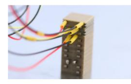
The Noliac shear stack NAC3402-H7.4 features motion in the X/Y/Z-axis. NAC3402-H7.4 measures 5x5 mm with a height of 7.4 mm and provides free stroke of 1.5/1.5/1.5  $\mu m$  and a capacitance of 0.8/0.8/5.5 nF.
