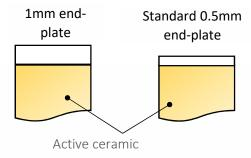
It is not possible to produce shear stacks without end-plates, as it would expose the live electrodes.
