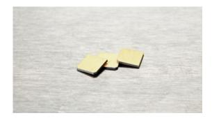
The Noliac shear plate actuators are characterized by providing a large stroke for a very compact design. The shear plate CSAP04 measures 15x15x0.5 mm and provides a free stroke of 1.5  $\mu$ m and a capacitance of 7.47 nF.
