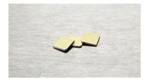
The Noliac shear plate actuators are characterized by providing a large stroke for a very compact design. The shear plate CSAP03 measures  $10 \times 10 \times 0.5$  mm and provides a free stroke of 1.5  $\mu$ m and a capacitance of 3.321 pF.
