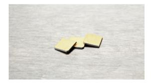
The Noliac shear plate actuators are characterized by providing a large stroke for a very compact design. The shear plate CSAP01 measures 2x2x0.5 mm and provides a free stroke of 1.5 µm and a capacitance of 133 pF.
