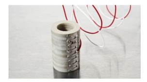
Noliac ring stack actuator NAC2123-Hxx (height in mm – Hxx) is based on the multilayer actuator NAC2123 and can be stacked to match you requirements. The standard range of NAC2123-Hxx is produced in a height between 4-120 mm. The ring stack provides a stroke in a range between 3.3 and 194.7  $\mu$ m and blocking force up to 3560 N depending on the height of the stack.
