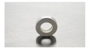
The Noliac piezo actuators can reach full performance at very low operating voltage. The ring actuator NAC2122 is 8x3 mm and provides a free stroke of  $3.3 \mu$ m and a blocking force of 1810 N.
