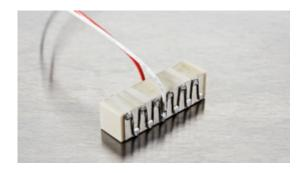
Noliac plate stack actuator NAC2021-Hxx (height in mm – Hxx) is based on the multilayer actuator NAC2021 and can be stacked to match you requirements. The standard range of NAC2021-Hxx is produced in a height between 4-70 mm. The plate stack provides a stroke up to 112.2  $\mu$ m and blocking force up to 2060 N depending on the height of the stack.
