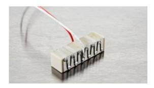
Noliac plate stack actuator NAC2011-Hxx (height in mm – Hxx) is based on the multilayer actuator NAC2011 and can be stacked to match you requirements. The standard range of NAC2011-Hxx is produced in a height between 4-20 mm. The plate stack provides a stroke up to 25.25  $\mu m$  and blocking force up to 168 N depending on the height of the stack.
