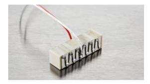
oliac plate stack actuator NAC2002-Hxx (height in mm – Hxx) is based on the multilayer actuator NAC2002 and can be stacked to match you requirements. The standard range of NAC2002-Hxx is produced in a height between 4-30 mm. The plate stack provides a stroke up to 39.9 µm and blocking force up to 378 N depending on the height of the stack.
