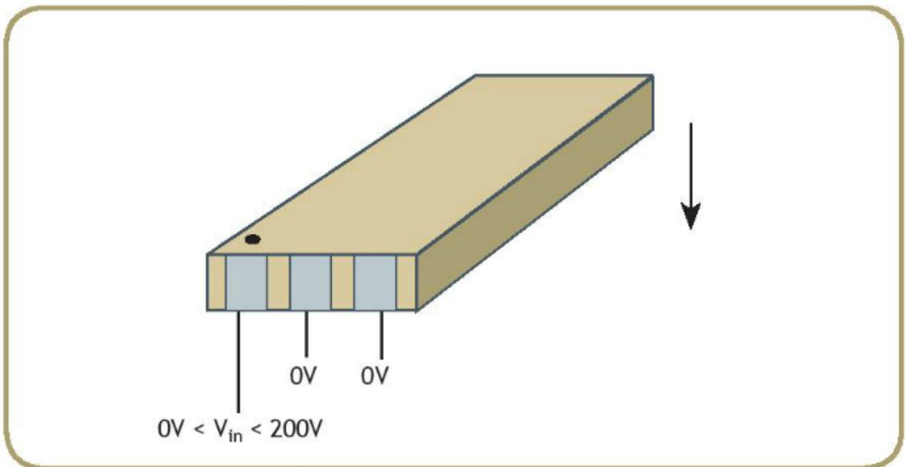
Noliac attaches these wires as standard to our plate and ring benders:
