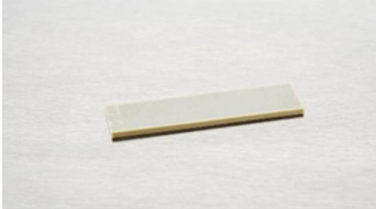
Noliac plate benders are manufactured with ceramic layer thickness down to 67 $\mu$ m as standard to facilitate very low operating voltage for full performance of the piezo material. CMBP08 measures 50x7.8x1.3 mm. The plate bender provides a stroke of +/- 850  $\mu$ m and a blocking force of 1.6 N.
