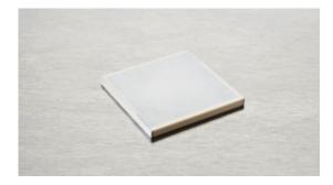
The multilayer piezo actuators can reach full performance at very low operating voltage. The plate actuator NAC2025 is 5x5 mm and provides a free stroke of 1.9  $\mu$ m and a blocking force of 800 N.
