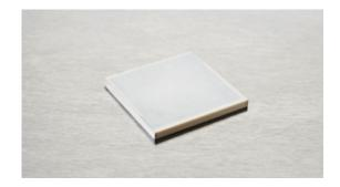
The multilayer piezo actuators can reach full performance at very low operating voltage. The plate actuator NAC2012 is 3x3 mm and provides a free stroke of  $3.3~\mu m$  and a blocking force of 378~N.
