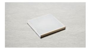
The multilayer piezo actuators can reach full performance at very low operating voltage. The plate actuator NAC2003 is 5x5 mm and provides a free stroke of 3  $\mu$ m and a blocking force of 1050 N.
