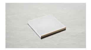
The multilayer piezo actuators can reach full performance at very low operating voltage. The plate actuator NAC2002 is 3x3 mm and provides a free stroke of  $3~\mu m$  and a blocking force of 378~N.
