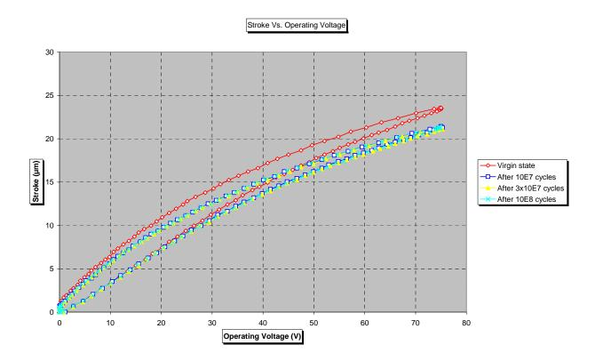
Upon request Noliac can supply "pre-aged" actuators that have been driven dynamically up to 10E7 cycles.
