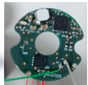
Fig. 5.o: Rotary shutter and its electronic printed circuit board Ø21.5mm
