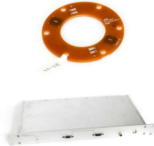
Fig. 9.n: EUCLID-NISP top counter sensor and associated electronics
