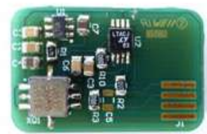
Fig. 9.k: Three axes accelerometer PCB mounted
