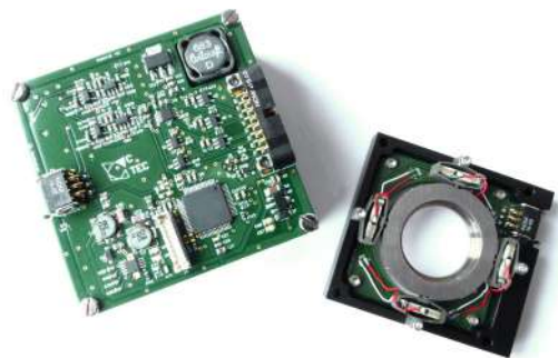
Fig. 7.r: Micro scanning piezo XY stage ( \pm 10 \mu\text{m} stroke) and its driver box for image resolution enhancement
