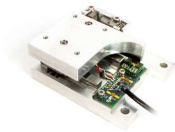
Fig. 5.f: MSPS35XS linear stage
