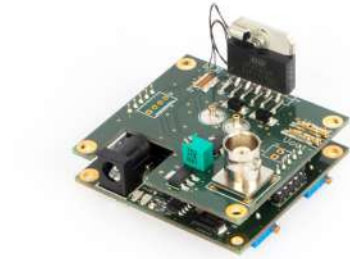
Fig. 8.x: OEM amplifier board for driving magnetic actuators
