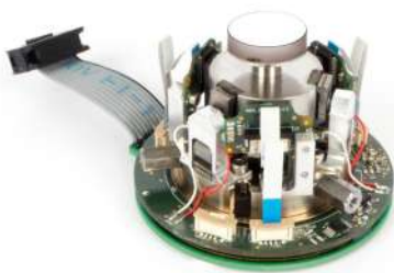
Fig. 3.ae: Tripod mechanism based on 3 piezo motors
