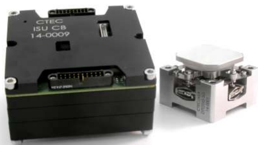
Fig. 7.p: Piezo FSM ( \pm 1 \text{ mrad} stroke) and its controller box for fine laser pointing & stabilization
