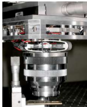
Fig. 3.f: XYZ200M-SG stage for IR Spectroscopy (courtesy of GES Lab / Montpellier University)
