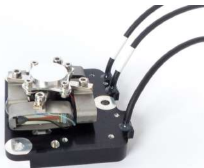
Fig. 5.k: Piezo FSM (+/- 1 mrad stroke) and its controller box for fine laser pointing & stabilisation
