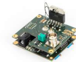
Fig. 8.v: OEM amplifier board for driving magnetic actuators
