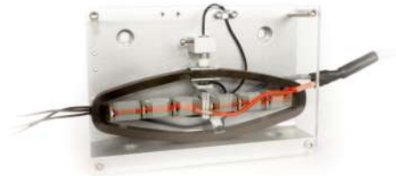
Fig. 4.c: ECP test bench for APA500L-CFRP-ECS
