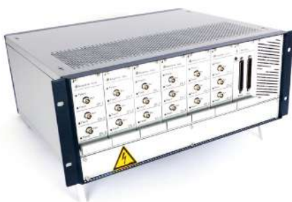
Fig. 9.u: 18 channels piezo emission rack
