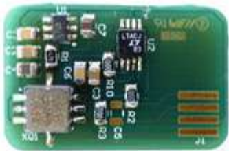
Fig. 9.l: Three axes accelerometer PCB mounted
