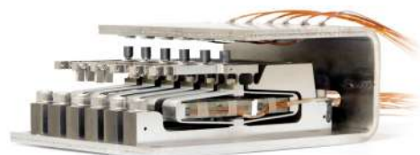
Fig. 5.m: Piezo activated arms (3 mm stroke) for X-ray filter holder 10 ms switching time
