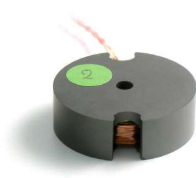
Fig. 9.p: PCI inductive sensor for MICHELIN MFP
