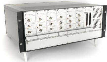
Fig. 8.n: 18 amplifier channels rack for high voltage piezo actuators
