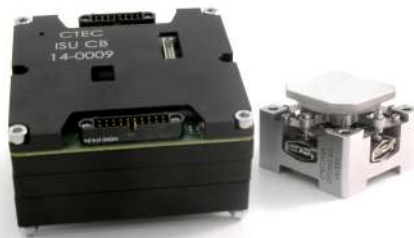
Fig. 5.k: Piezo FSM (+/- 1 mrad stroke) and its controller box for fine laser pointing & stabilisation
