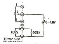
• If powered by external voltage source, instead of the speed control, connect to the DC variable power source as shown above. Instead of changing the voltage from 0~1.6V, by changing the volume from 0~max, similar speed control is possible.
