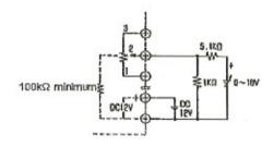
If you wish to expand the variable scope of external voltage, there is an electrical resistance partial pressure method.
