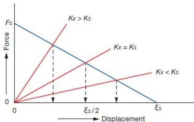
Fig. 2 Relation between load and generated displacement
