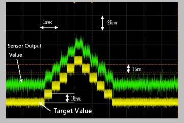
Achieved stable and high-precision positioning, against the 15nm increment target value.
